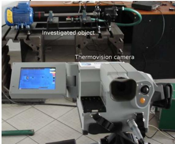
Fig. 2. Investigated object and applied infrared camera
