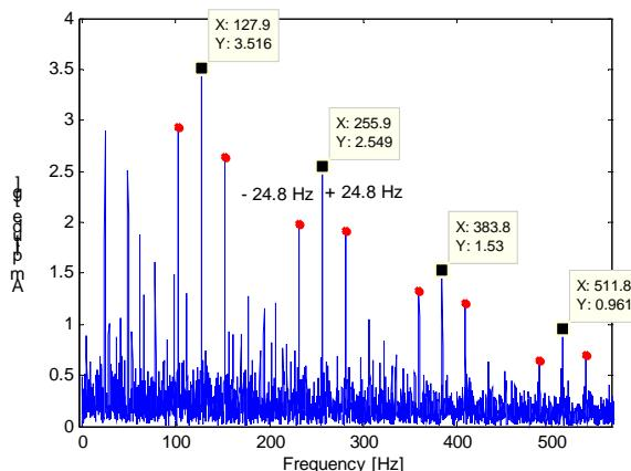
Rys. 9. Narrowband envelope spectrum ( $CF=8900$  Hz,  $dF=600$  Hz)
