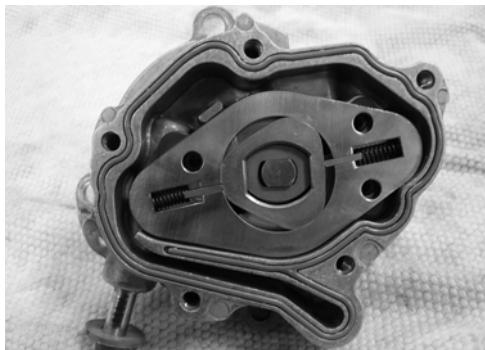
Fig. 2. Negative-pressure pump (fuel pump is on other side)
