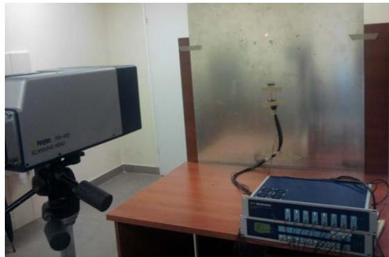
Fig. 9. Experimental setup for phased array testing.
