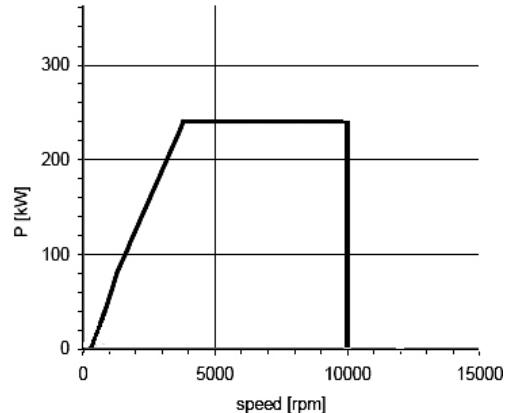
Fig. 8. Power characteristic of test brake
