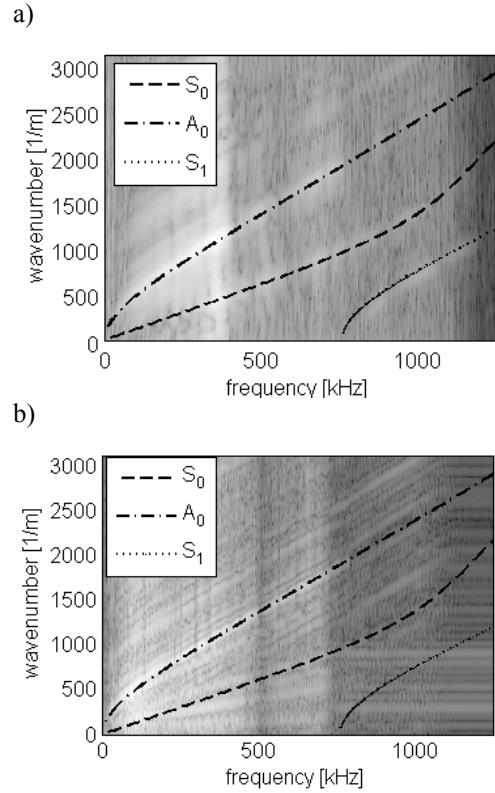
Fig. 5. Theoretical and measured wavenumber vs. frequency plot obtained for signals acquired by
