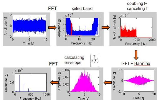
Fig. 7 The algorithm of envelope spectrum generation [1]
