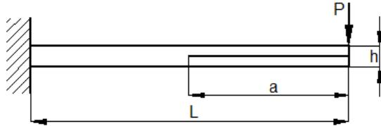
Fig. 1. Configuration of ELS plate
