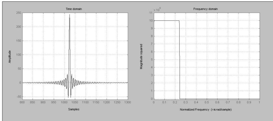
Fig. 12. Spectrum of FPR filter generated by Remez algorithm after windowing with Blackman window
