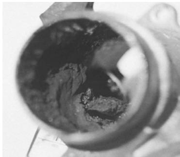
Fig. 5: Gummed up intake valve of EGR [4]
