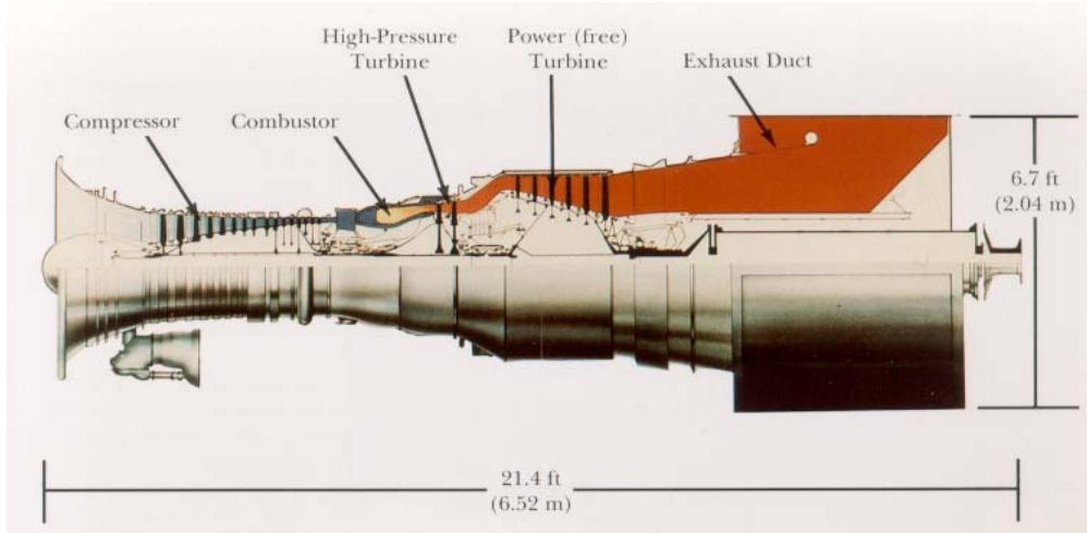
Fig. 2. Longitudinal cross-section of examined L-2500 engine
