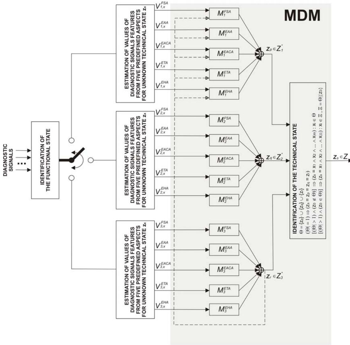
Fig. 5. The structure of the multispect diagnostic model (MDM)
