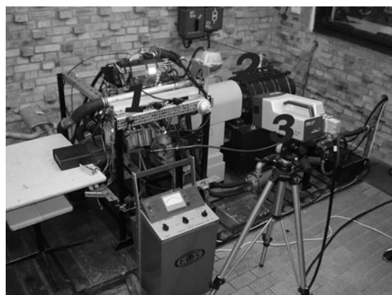
Fig. 6. Measuring rig: engine (1), electrorotary brake (2), vibrometeric head (3)
