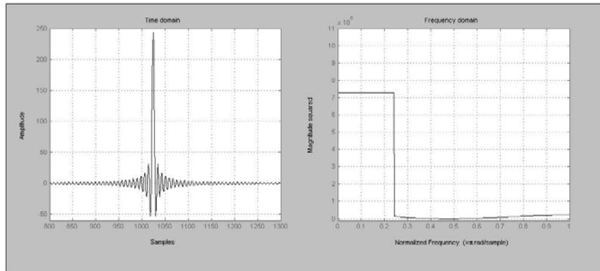
Fig. 11. Spectrum of FPR filter generated by Remez algorithm
