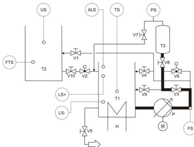
Fig. 2. Compression of air in the tank T3 by water flowing from the tank T1 to the tank T3 (bold curve shows the flow of water)
