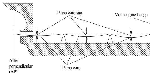
Fig. 1. Example of shafting alignment using piano wire
