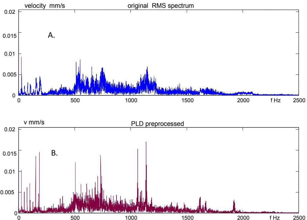
Fig. 3. Run – out of L-2500 ,vibration spectraPLD equalized:
