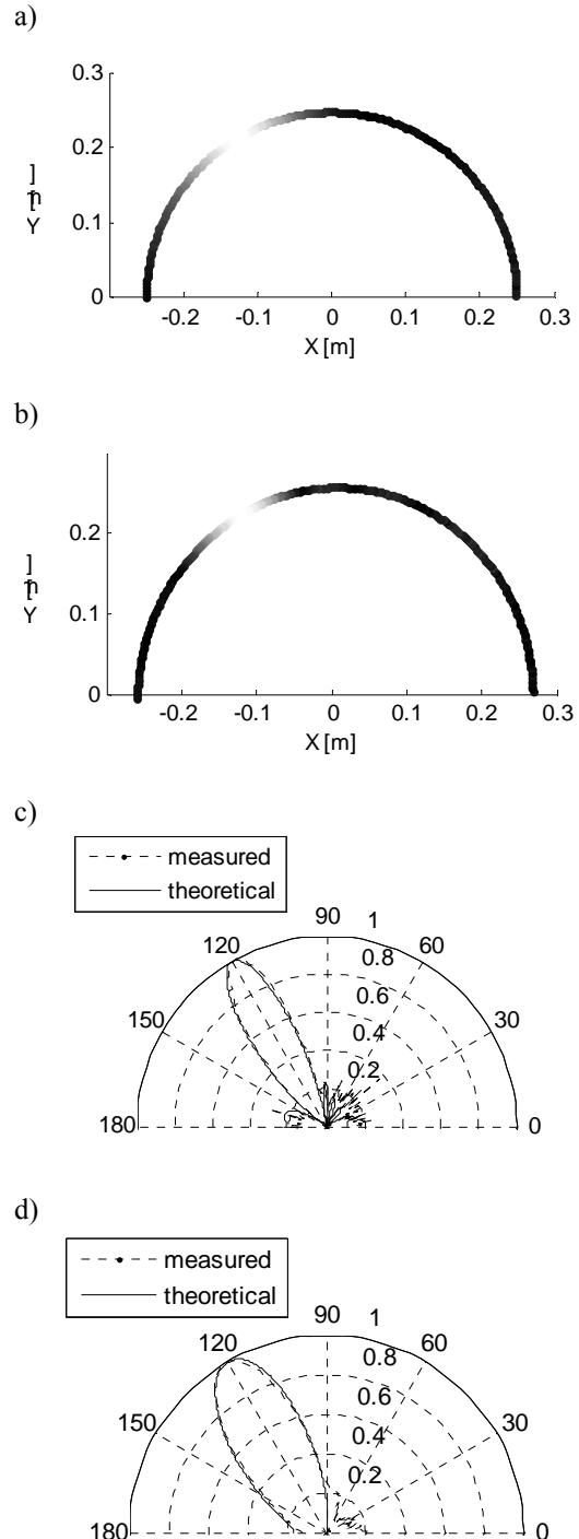
Fig. 10. Measurement points and amplitude values- a) linear apodization b) Hamming apodization.
