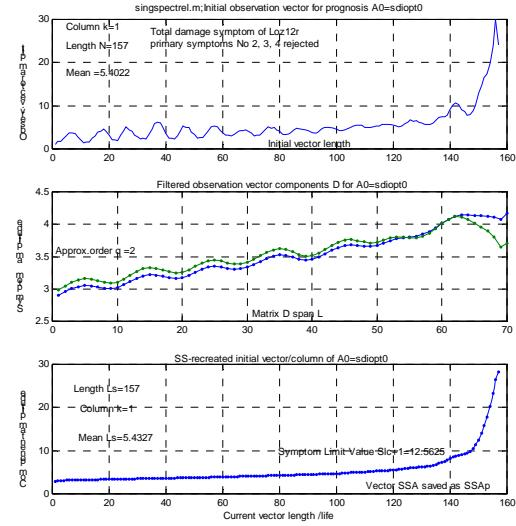
Fig. 5. Denoised total damage symptom of a rolling bearing testing rig with pulsating load
