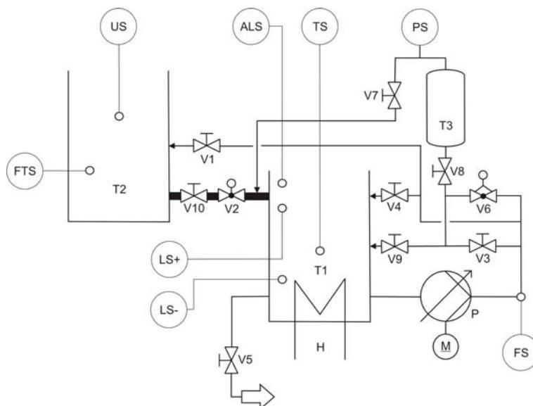
Fig. 3. Filling the tank T1 by water from the tank T2 (bold line shows the flow of water)
