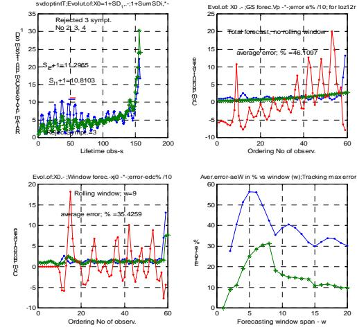
Fig. 4. GST forecast of a symptom value (first generalized symptom), with and without rolling window, for the ball bearing test rig (see Fig. 3)
