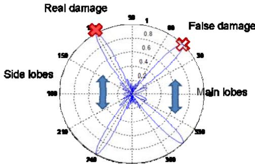
Fig. 8. "False damage" effect.
