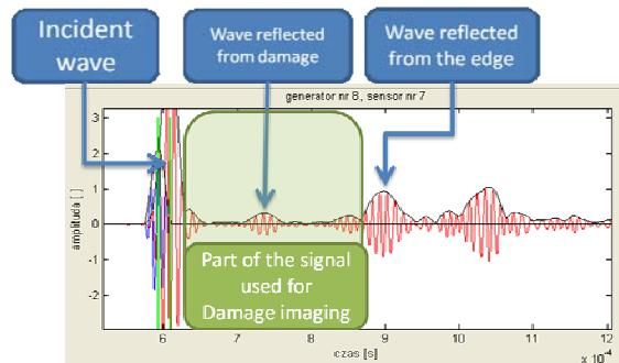
Fig. 6. Example of structure response signal with damage.
