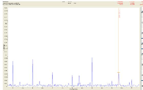
Fig. 6. High-resolution envelope spectrum. Two lines caused by the inner bearing fault are visible
