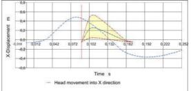
Fig. 7. Horizontal head displacements of a manmodel and displacements of a multi-section air headrest at activation time t=0.090s
