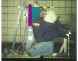
Fig. 3. The concept of the functioning of head back and spine ideal protection – 3 upper sections activated
