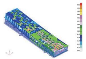
Fig. 5. Reduced stress (by H-M-H11) [MPa] and the displacement in the model wing. The apparent local loss of stability
