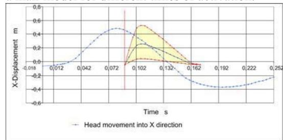
Fig. 7. Horizontal head displacements of a man-model and displacements of a multi-section air headrest at activation time  $t=0.090$ s
