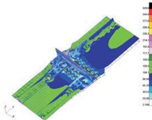
Fig. 6. The combination of riveting, a local model of the wing - reduced stress (by H-M-H) [MPa] - frame and cover on the side of formed rivet heads
