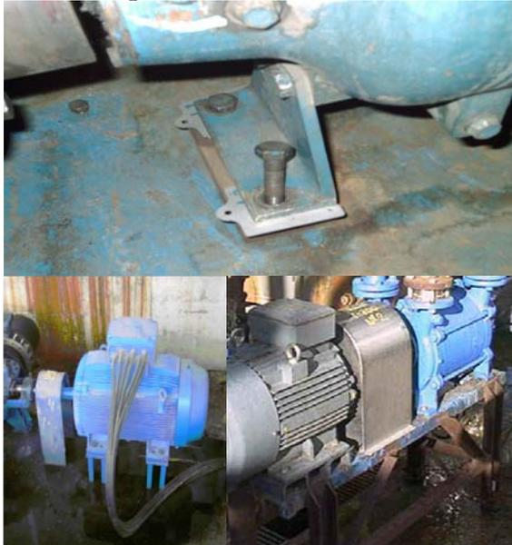
Fig. 5. Rotating machines with a weak bench
