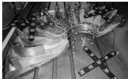
Fig. 2. Diaphragm during the optical measurement
