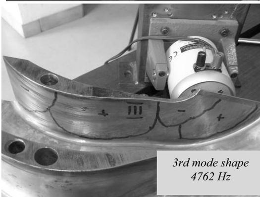
Fig. 6. Experimental and model natural frequencies of diaphragm vane No.1. in response to the white noise excitation
