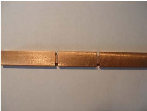
Fig. 3. A specimen with a P-type notch
