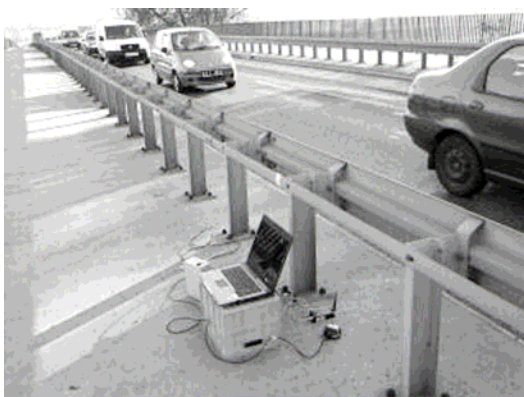
Fig. 11. Measuring set-up during modal testing of a bridge span
