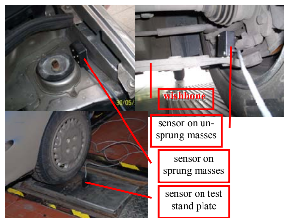
Fig. 2. Elements of measurement system
