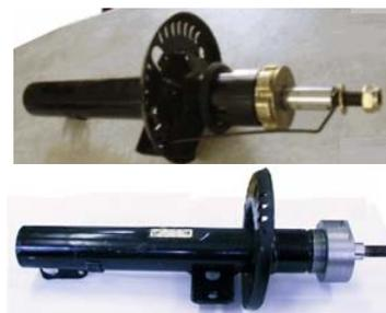
Fig.1. The shock absorber before and after modification
