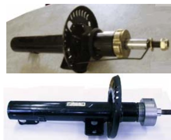
Fig.1. The shock absorber before and after modification
