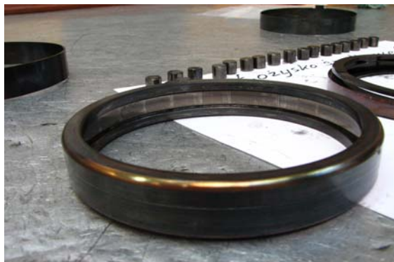
Fig. 9. Resonance impression on outside race of the rolling bearing
