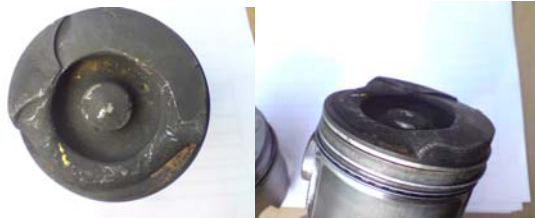
Fig. 4. Failure of the valve due to long-lasting exploitation with broken injectors
