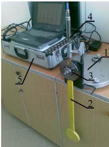
Fig. 3. A view of the test stand for identification of the technical condition of a rolling bearing. 1 – base with a holder, 2 – test pendulum, 3 – tested bearing, 4 – photo-optical sensor, 5 – recording device KSD-400
