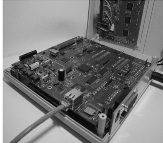
Fig. 3. PCB board and electronic devices view of the PUD
