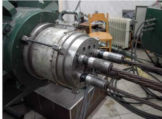
Fig. 9. View of the fasten of force sensors
