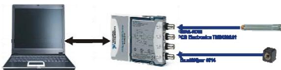
Fig. 2. The measurement equipment
