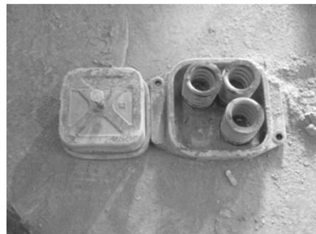
Fig. 1. An example of springy vibroisolator
