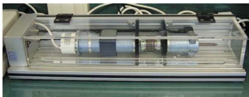
Fig. 2. Laboratory stand with a DC engine
