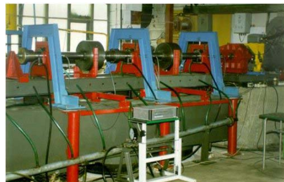
Fig. 3. Multi-scale research rig used for experimental verification of NLDW system. The object assumed in further investigations.
