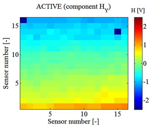
Fig. 25. Distribution of  $H_y$  component of the magnetic field on the surface of the homogeneous sample (without the welded joint)
