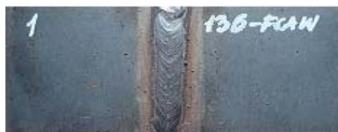
Fig. 3. The welded joint made by MAG method
