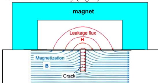
Fig. 1. Magnetic flux leakage at the location of a crack
