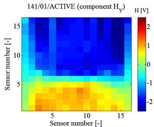
Fig. 23. Distribution of  $H_y$  component of the magnetic field on the surface of the faulty sample 141/01
