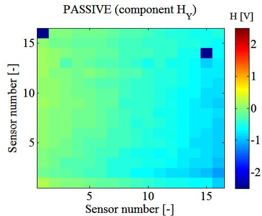
Fig. 16. Distribution of  $H_y$  component of the magnetic field on the surface of the homogeneous sample (without welded joint)
