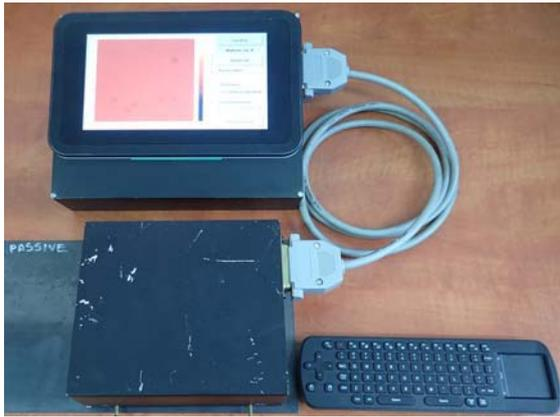
Fig. 8. Measurement instruments used for passive magnetic tests
