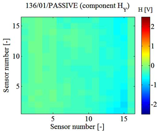
Fig. 14. Distribution of  $H_y$  component of the magnetic field on the surface of the faulty sample 136/01
