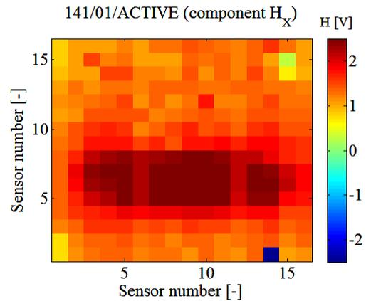
Fig. 22. Distribution of  $H_x$  component of the magnetic field on the surface of the faulty sample 141/01
