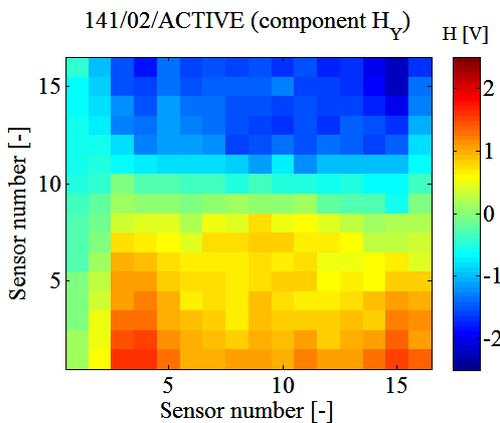
Fig. 21. Distribution of  $H_y$  component of the magnetic field on the surface of the reference sample 141/02
