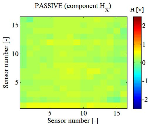
Fig. 15. Distribution of  $H_x$  component of the magnetic field on the surface of the homogeneous sample (without welded joint)
