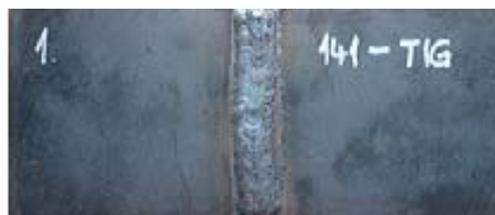
Fig. 4. The welded joint made by TIG method
