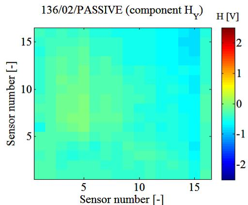
Fig. 12. Distribution of  $H_y$  component of the magnetic field on the surface of the reference sample 136/02
