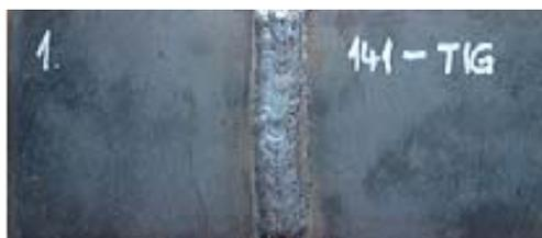
Fig. 4. The welded joint made by TIG method
