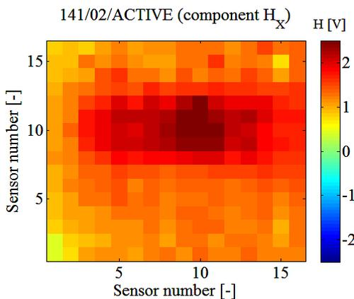
Fig. 20. Distribution of  $H_x$  component of the magnetic field on the surface of the reference sample 141/02
