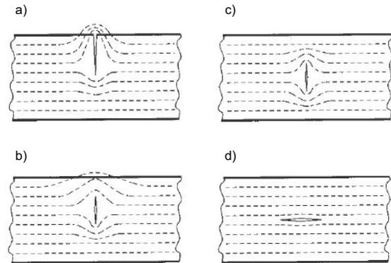
Fig. 2. Influence of material's inhomogeneity location and orientation on the magnetic flux leakage effect:
