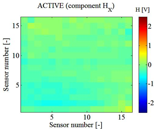
Fig. 24. Distribution of  $H_x$  component of the magnetic field on the surface of the homogeneous sample (without the welded joint)
