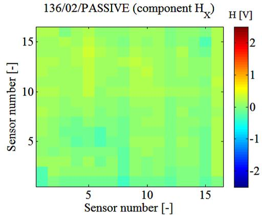
Fig. 11. Distribution of  $H_x$  component of the magnetic field on the surface of the reference sample 136/02
