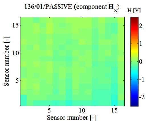
Fig. 13. Distribution of  $H_x$  component of the magnetic field on the surface of the faulty sample 136/01
