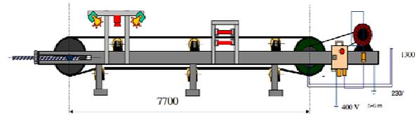
Fig. 5. Test stand for the diagnostics of conveyor belts
