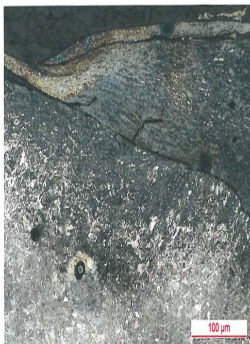
Fig. 4. The cracks in samples of the material collected from the bottom part of the track groove. In the upper part is the sample 4A, in the lower part is the sample 7A
