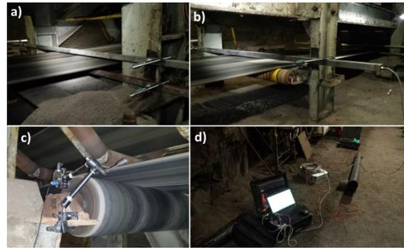
Fig. 1. DIAGBELT system mounted on the investigated conveyor; a) permanent magnet bars, b) magnetic head, c) tachometer, d) data acquisition module and a portable computer with the software
