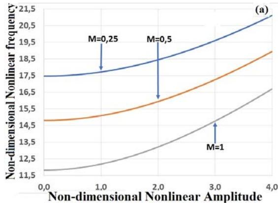
Fig. 7(a) First nonlinear mode Backbone curves for various values of the mass located at the middle
