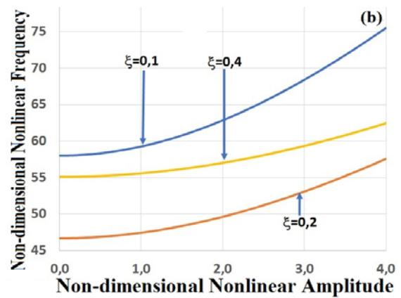
Fig. 7(b) second nonlinear mode Backbone curves for various locations of the mass  $M=0.5$
