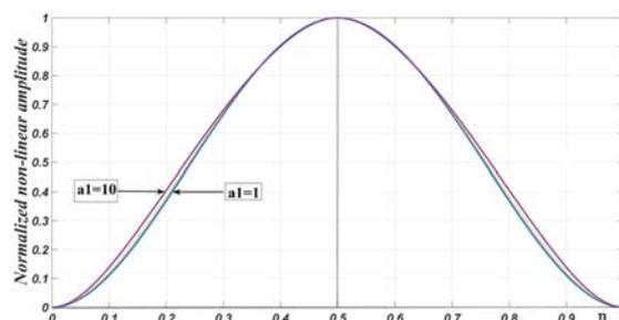
Fig. 10. The normalized first non-linear mode shape of a CBA05PM ( $M=0.5$  and  $\xi=0.5$ )
