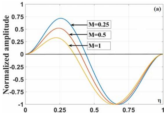
Fig. 6(a) Second normalized linear mode shape for various values of the mass located at the quarter of the beam ( $u=L/4$ )
