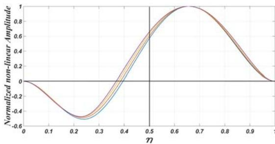
Fig. 14. The normalized non-linear second mode shapes ( $M=0.5$  and  $\xi=0.25$ )
