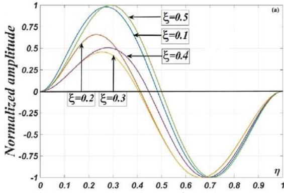
Fig. 5(a) Second mode shape for various mass locations and  $M=0.5$
