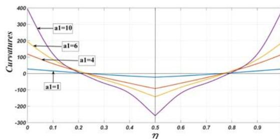
Fig. 11. The first non-linear curvatures of the CBAPM ( $M=0.5$  and  $\xi=0.5$ )
