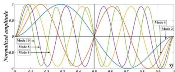
Fig. 9. Anti-symmetrical CBA05PM linear mode shapes for  $i=2,4,6,8,10$  ( $M=0.5$  and  $\xi=0.5$ )
