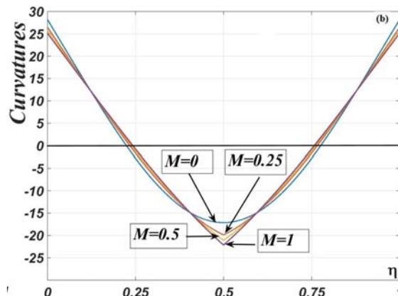
Fig. 4(b) Curvatures associated to the first mode for various values of the mass located at the middle of the beam ( $u=L/2$ ).
