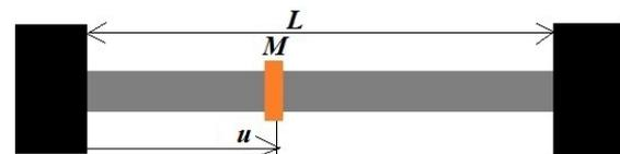
Fig. 1. The clamped beam with a point mass
