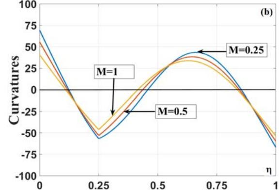
Fig. 6(b) Curvatures associated to the second mode for various values of the mass located at the quarter of the beam ( $u=L/4$ )
