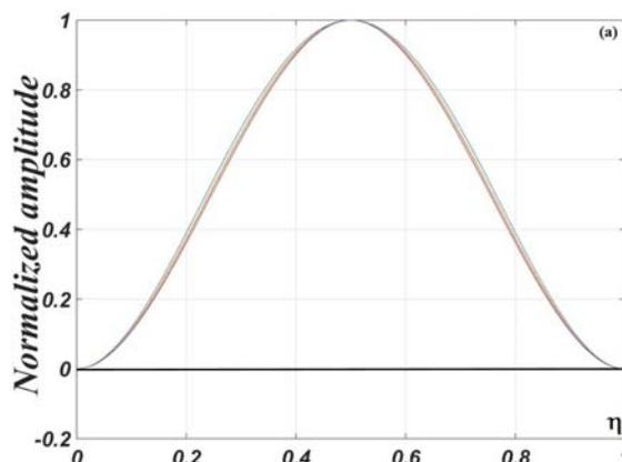
Fig. 4(a) First normalized mode shape for various values of the mass located at the middle of the beam ( $u=L/2$ ).
