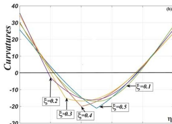
Fig. 3(b) Curvatures associated to the first mode shape for  $M = 0.5$  at various locations.
