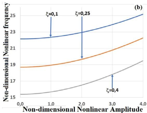
Fig. 7(b) First nonlinear mode Backbone curves for various locations of the mass  $M=0.5$
