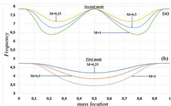
Fig. 2 Effect of the added mass location on the linear frequencies associated to (a) the first mode (b) the second mode, for  $M = 0.25, 0.5$  and  $1$
