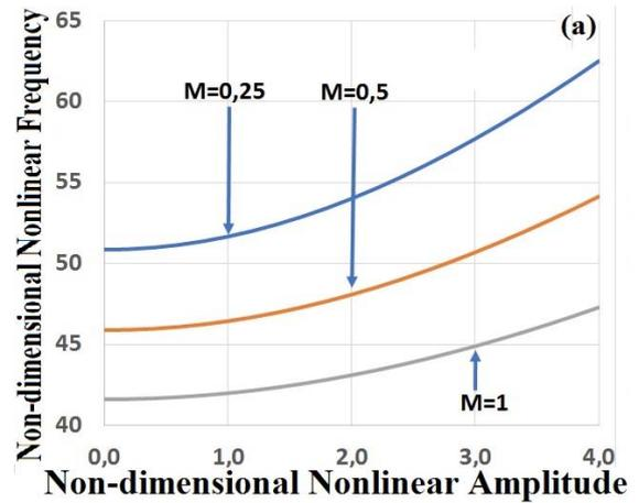
Fig. 8(a) Second nonlinear mode Backbone curves for various values of the mass located at the middle
