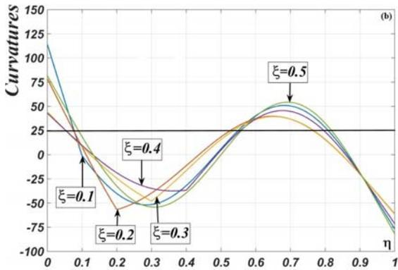
Fig. 5(b) Curvatures associated to the second mode for various mass locations and  $M=0.5$
