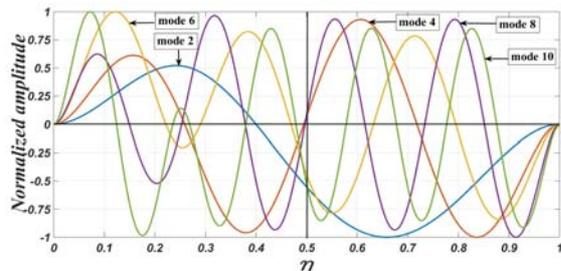
Fig. 13. Anti-symmetrical CBA0.25PM functions for  $i=2,4,6,8,10$  ( $M=0.5$  and  $\xi=0.25$ )
