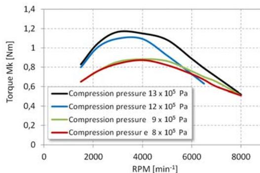
Fig. 7. Torque in relation to revolutions measured at various compression pressures
