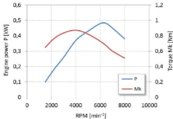
Fig. 9. Measured engine power and torque after 120 minutes of engine operation
