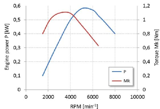
Fig. 8. Measured engine power and torque at optimal engine operation
