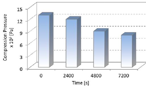
Fig. 4. Engine compression pressure values
