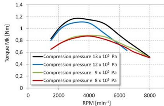
Fig. 7. Torque in relation to revolutions measured at various compression pressures
