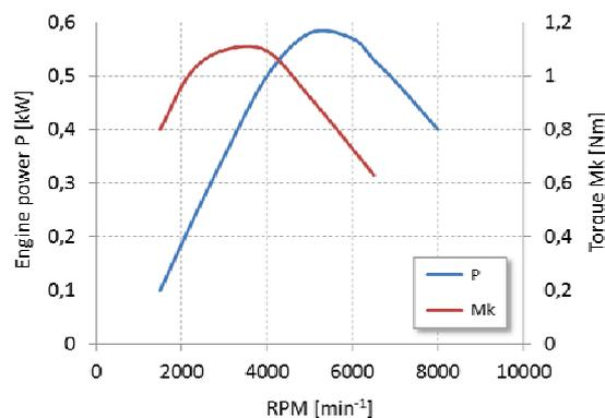
Fig. 8. Measured engine power and torque at optimal engine operation
