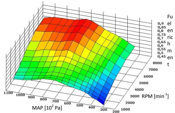
Fig. 2. Power measurement fuel 3D map
