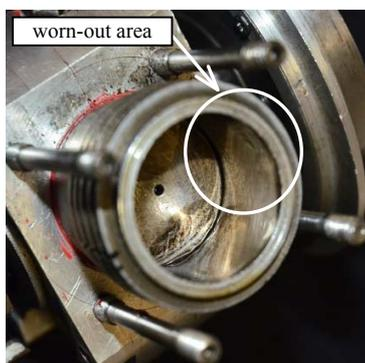
Fig. 11. Cylinder wall wear
