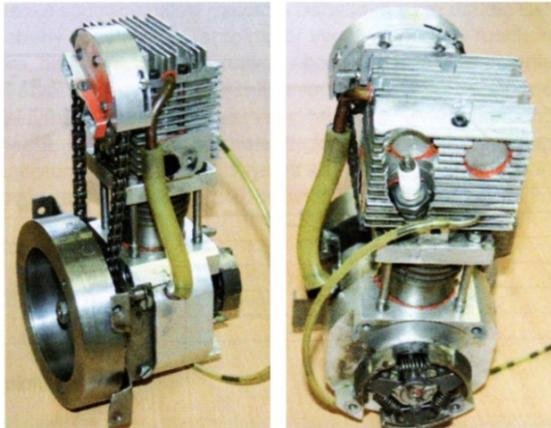
Fig. 1. Experimental combustion engine [15]
