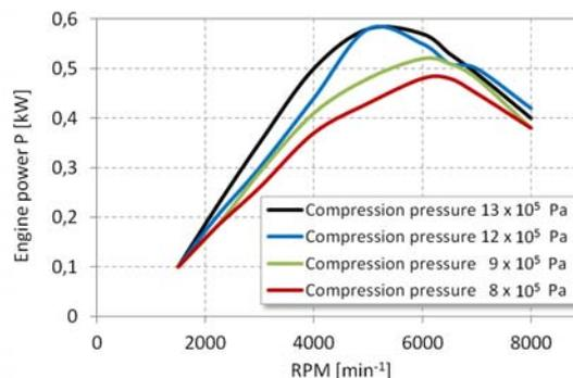
Fig. 6. Engine power in relation to the revolutions measured at various compression pressures
