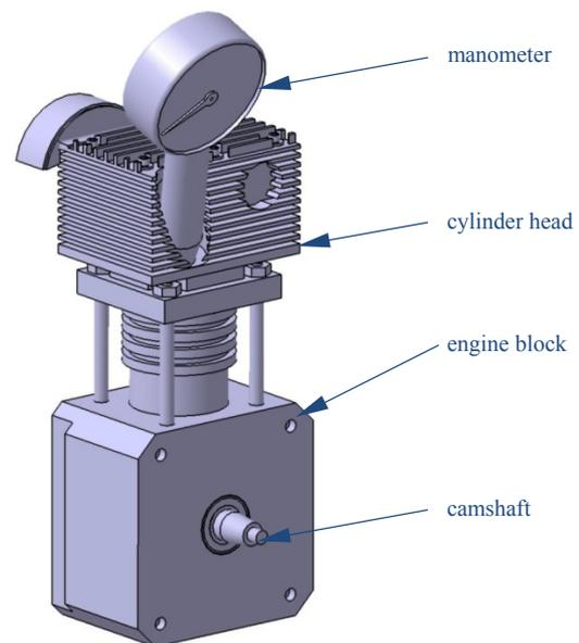
Fig. 3. Compression pressure measuring model
