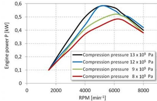
Fig. 6. Engine power in relation to the revolutions measured at various compression pressures
