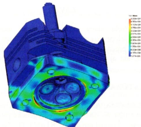
Fig. 12. Bending stresses on the installation surface of the cylinder head [15,18]
