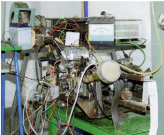
Fig. 5. Dynamometer and the prototype engine [15,18]
