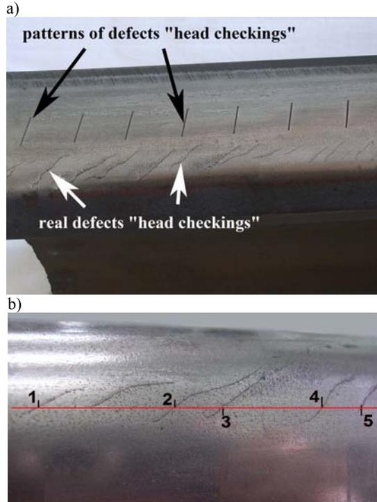
Fig. 1. The tested rail: a) with patterns and real defects, b) with scan way on real disadvantages signed in turn from 1 to 5
