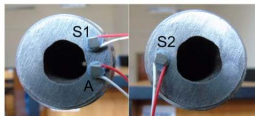
Fig. 6. PZT transducers at the single self-drilling hollow bar: a) configuration of actuator and sensors; b) detail showing actuator and sensors at the beginning and the end of the bar
