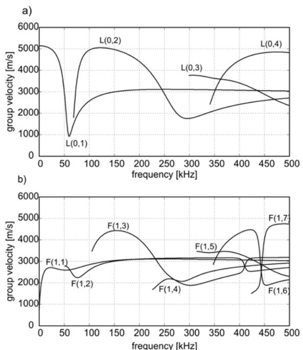
Fig. 3. Dispersion curves for steel hollow bar ( $E = 210$  GPa,  $\nu = 0.3$ ,  $\rho = 7938.54$  kg/m<sup>3</sup>) with external diameter of 38 mm and internal diameter of 19 mm: a) longitudinal modes, b) flexural modes
