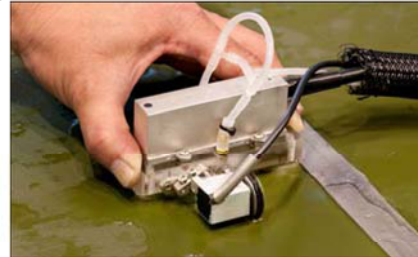
Fig. 9. An example of UT-PA testing head [9]
