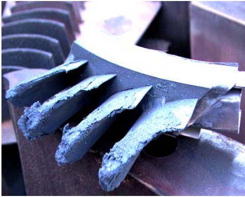
Fig. 8. Wear of the fins of a gas turbine
