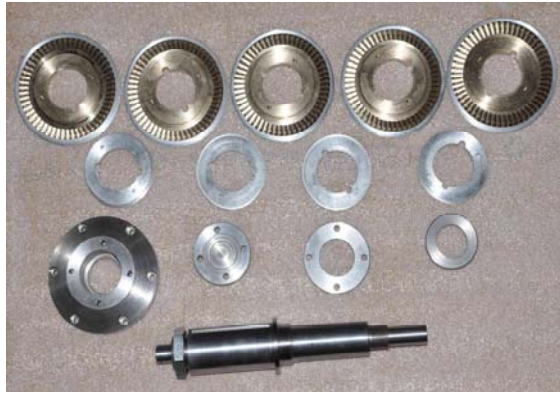
Fig. 3. Photo showing the shaft, microturbine rotors, bearing casing and packing rings of the microturbine [37]
