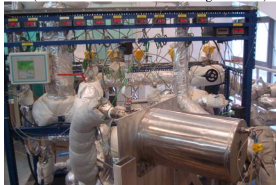
Fig. 2. Axial-flow microturbine connected with the ORC system [37]
