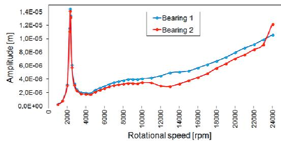
Fig. 13. Vibration amplitudes of the bearing journals (variant no. 4).
