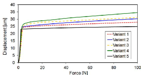
Fig. 5. Structural stiffness of a supporting layer for five different foil bearings.
