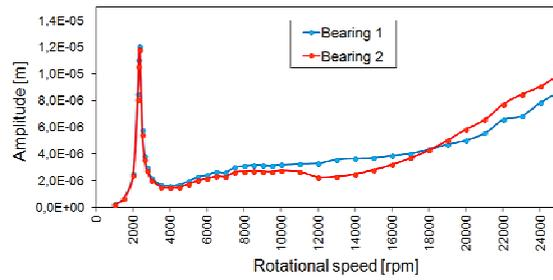
Fig. 9. Vibration amplitudes of the bearing journals (variant no. 2).
