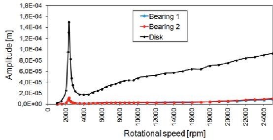
Fig. 8. Vibration amplitudes of the bearing journals and of the disk (variant no. 2).
