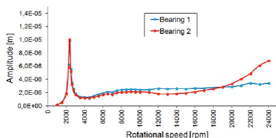
Fig. 15. Vibration amplitudes of the bearing journals (variant no. 5).
