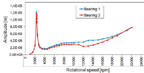
Fig. 11. Vibration amplitudes of the bearing journals (variant no. 3).
