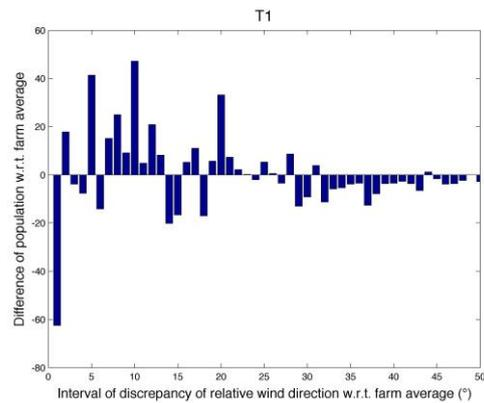
Fig. 10. Difference in distribution of relative wind direction with respect to the farm average, T1. D2 data set.
