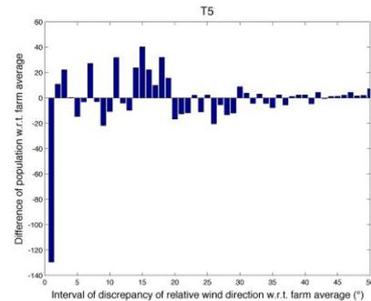
Fig. 9. Difference in distribution of relative wind direction with respect to the farm average, T5. D2 data set.
