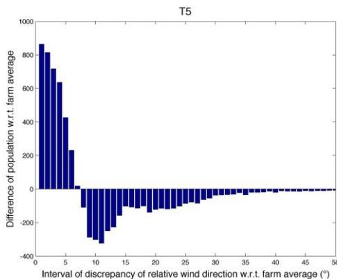
Fig. 4. Difference in distribution of relative wind direction with respect to the farm average, T5. D1 data set.
