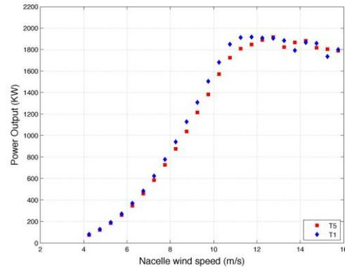
Fig. 2. Power curves of turbines T5 and T1. D1 data set, 0.5 m/s nacelle wind speed interval.
