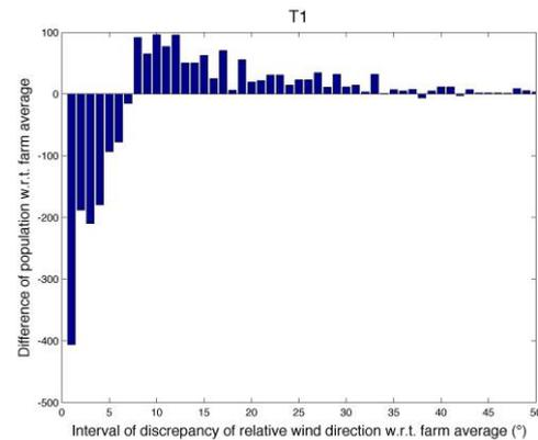
Fig. 5. Difference in distribution of relative wind direction with respect to the farm average, T1. D1 data set.
