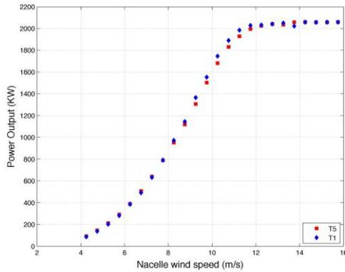
Fig. 7. Power curves of turbines T5 and T1. D2 data
