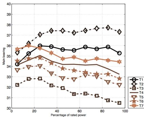
Fig. 4. Main bearing temperature vs Power, during the training period. Bins have amplitude of the 10% of the rated power
