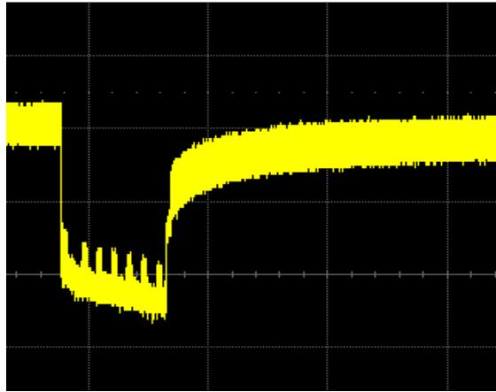
Fig. 3 Capacitor voltage signal during charging of capacitor for a longer period of time
