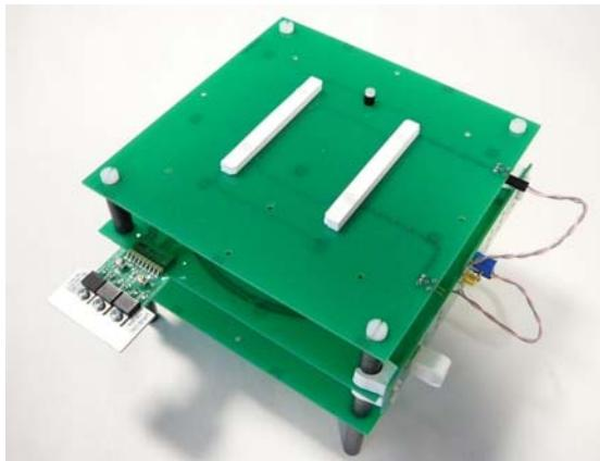
Fig. 1. ISO 10373-6 module connected to the external sine generator
