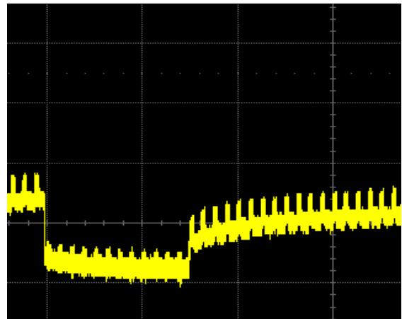
Fig. 5. Charging of capacitor in the field generated by the lowest-class antenna. The pooling problem is visible.
