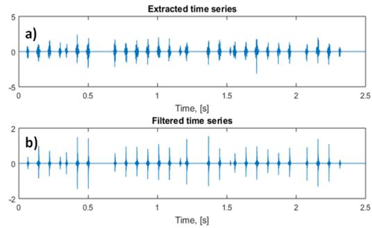
Fig. 5. Recovered time series: a) after ISTFT transformation from selected partial spectrogram, b) after further highpass filtration
