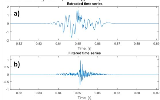
Fig. 6. Example of impulse shape before and after filtration
