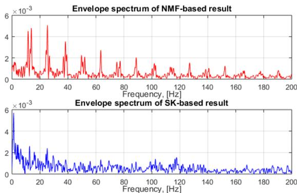
Fig. 9. Comparison of output signals' envelope spectra after SK filtration and after processing with our method
