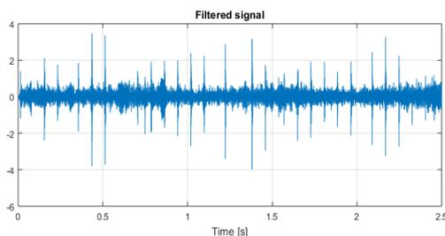
Fig. 8. Result of filtering using Spectral Kurtosis
