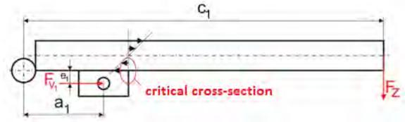
Fig. 7. Position of the considered critical cross section
