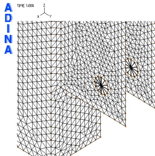
Fig. 20. Detail of the arm column mesh
