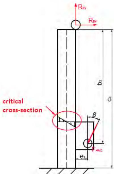
Fig. 17. Position of the considered critical cross section
