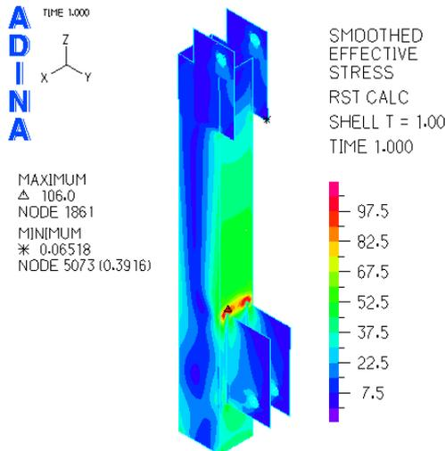
Fig. 21. Equivalent stress distribution in the column
