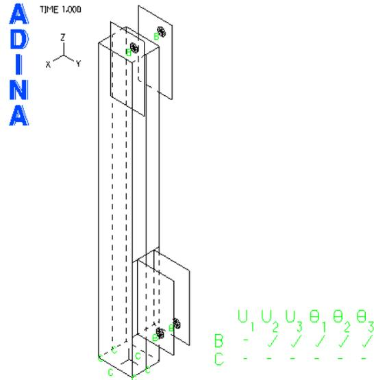
Fig. 18. Removing degrees of freedom of the column
