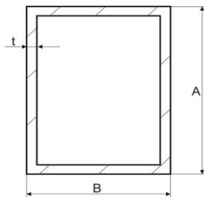
Fig. 3. The profile chosen for the hydraulic arm construction
