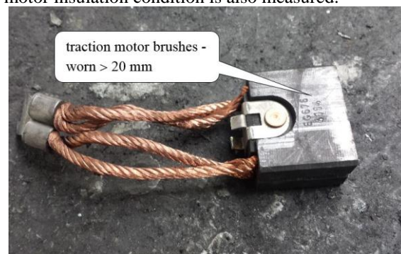
Fig. 8. Worn brushes traction motor
