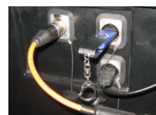
Fig. 1. USB (or DIN) slots for downloading of operational data
