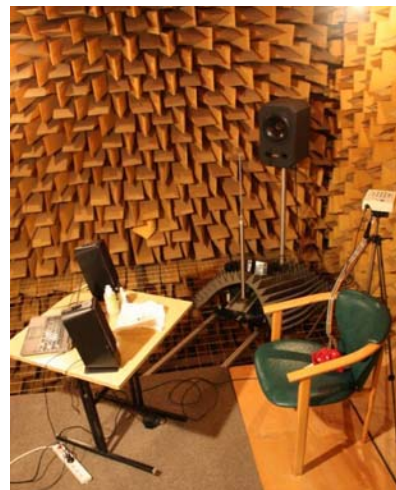
Fig. 1. Research setup in a small anechoic chamber to evaluate EEG of the volunteers during listening of recorded sounds
