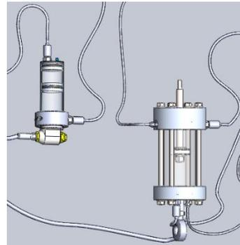
Fig. 3. Render of the transparent monotube shock absorber
