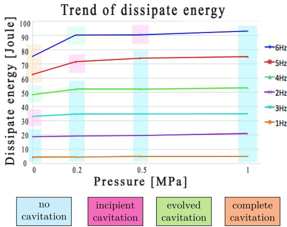
Fig. 14. Variation the performance of the shock absorber
