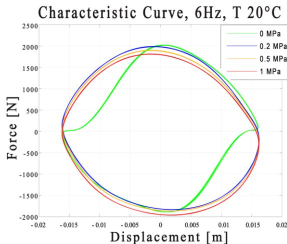
Fig. 5. Characteristic Curve, 6Hz, [0 - 0.2 - 0.5 - 1 MPa]
