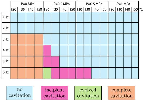
Fig. 10. Summary grid of an optical evaluation
