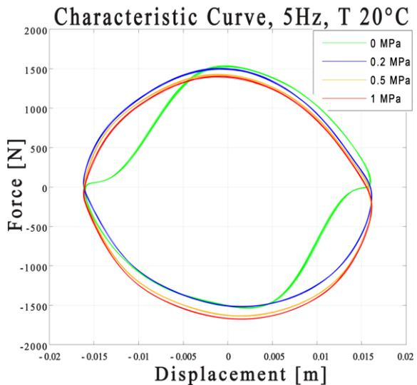
Fig. 9. Characteristic Curve, 5Hz, [0 - 0.2 - 0.5 - 1 MPa]
