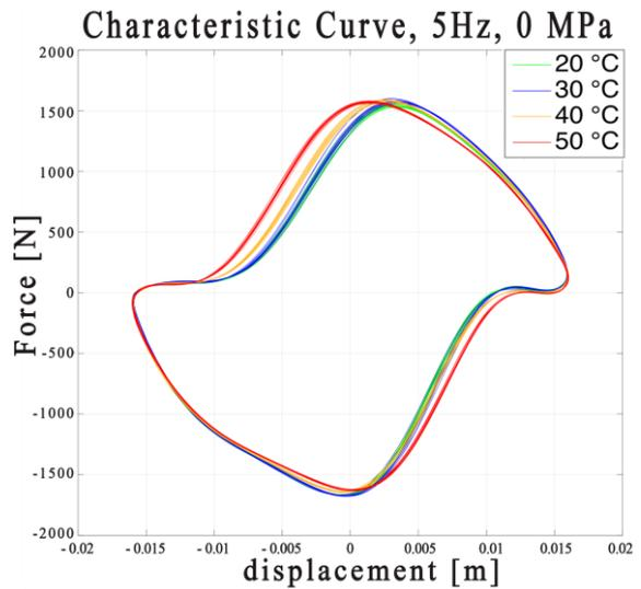
Fig. 13. Characteristic Curve, 5Hz, 0MPa, [20-30-40-50 °C]
