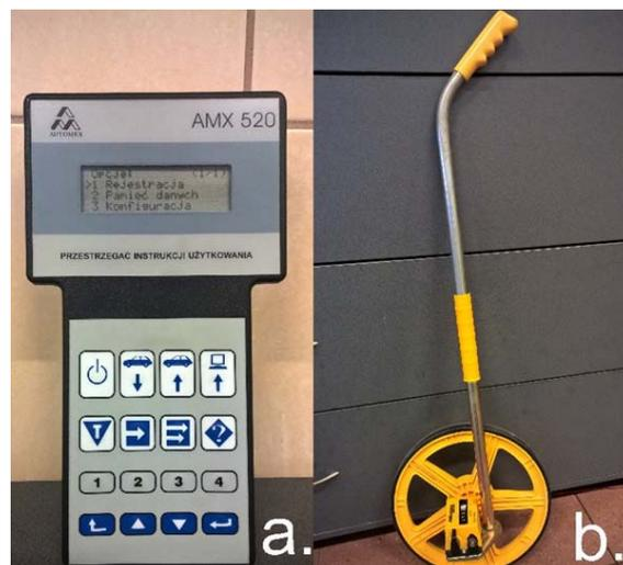
Fig. 4. Measuring instruments a) AMX 520 decelerometer and b) Trumeter 5500 road measuring wheel
