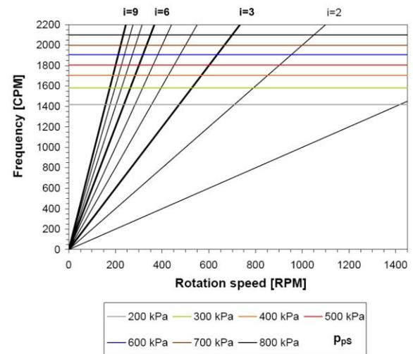
Fig. 7. The Campbell's diagram of the mechanical system
