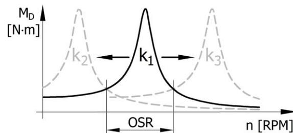
Fig. 1. Mechanical systems tuning principle
