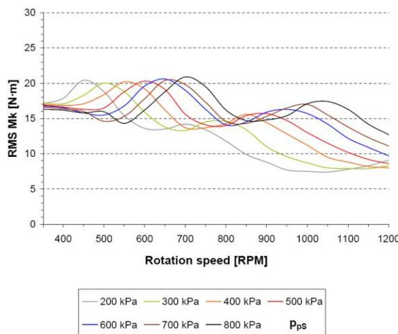
Fig. 8. Measured resonance curves of the mechanical system at one cylinder fall-out operation
