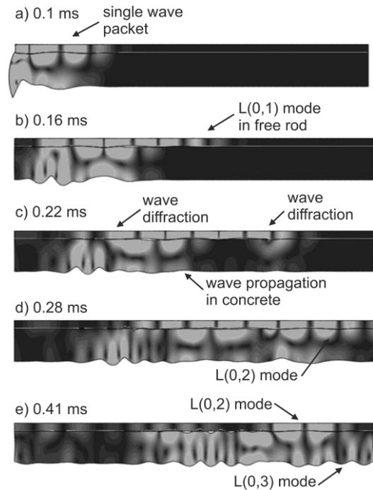
Fig. 15. Wave propagation in rod embedded in concrete cover with debonding at the middle part (model #4,  $L_f = 40$  cm)
