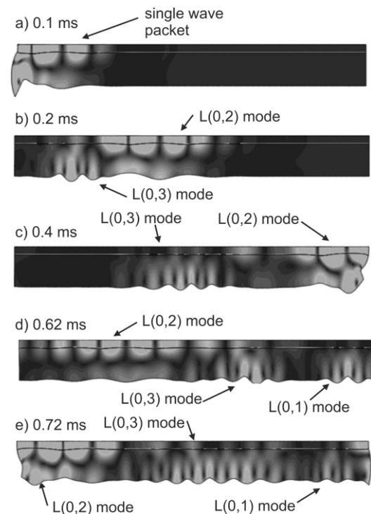
Fig. 9. Wave propagation in the rod perfectly bonded with concrete cover (model #2)
