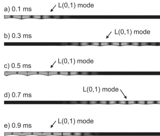
Fig. 8. Wave propagation in the free rod (model #1)
