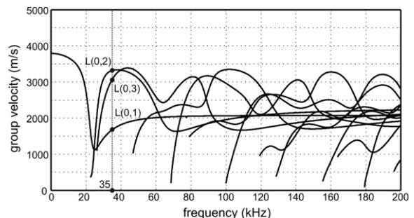
Fig. 2. Dispersion curves for a steel 2 cm diameter rod ( $E = 210$  GPa,  $\nu = 0.2$ ,  $\rho = 7820$  kg/m<sup>3</sup>) embedded in concrete cover with 4 cm thickness ( $E = 26$  GPa,  $\nu = 0.2$ ,  $\rho = 2084$  kg/m<sup>3</sup>)
