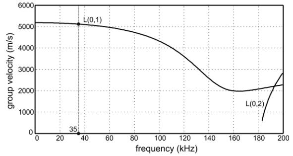
Fig. 1. Dispersion curves for a steel 2 cm diameter rod ( $E = 210$  GPa,  $\nu = 0.3$ ,  $\rho = 7820$  kg/m<sup>3</sup>)
