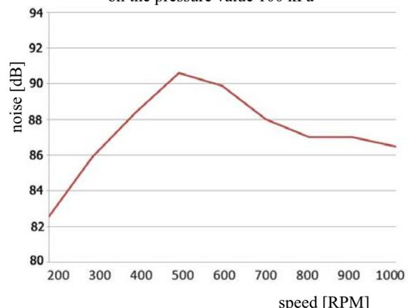
Fig. 6. Dependence of the speed on the noise level of the mechanical system using pneumatic coupling pressurized on the pressure value 100 kPa
