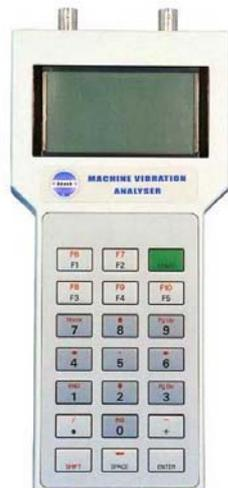
Fig. 4. Vibration analyzer Adash 4101
