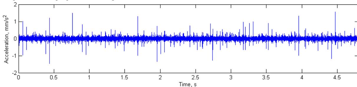
Fig.17. Time-domain representation of the analyzed signal of the rolling bearing with the fault
