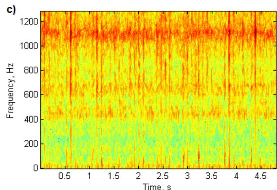
Fig.18. Spectrum of vibration signal of bearing obtained using a) reassigned spectrogram, b) reassigned PMHD, c) reassigned SPWVD
