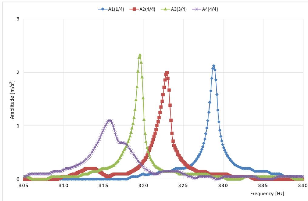
Fig. 2. The results of the FFT analysis of 12x4.25 wheel rims with a different number of weld joints between the rim and the disk (fragment of the spectrum).
