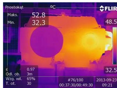
Fig. 5. Thermal image of the inspected gear system
