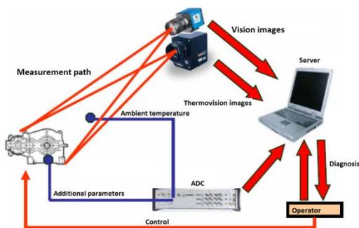
Fig. 3. Scheme of continuous thermal imaging diagnostics system [2]
