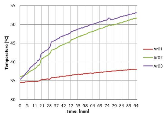
Fig. 11. Average temperature change for gear wheels (areas Ar01, Ar02, Ar03)
