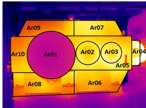
Fig. 9. Division of gear system into areas Ar
