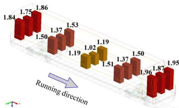
Fig. 10.  $N_{MV}$  indices for the speed of 85 km/h
