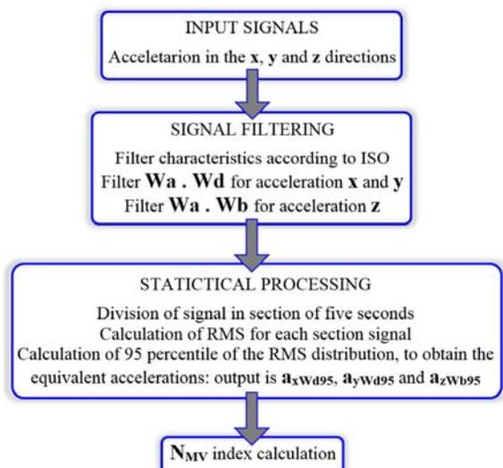
Fig. 5. Calculation process for  $N_{MV}$  comfort index
