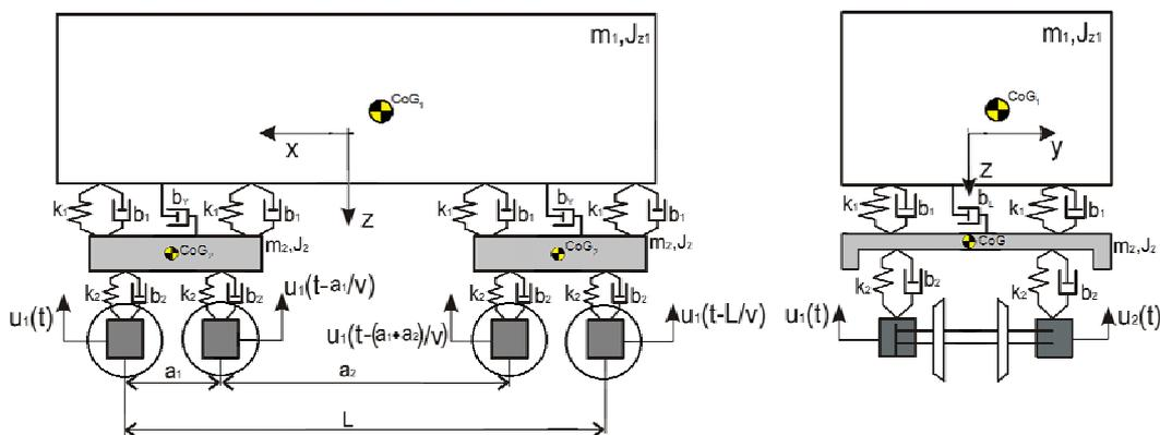
Fig. 1. Passenger car multibody system – dynamic schematic
