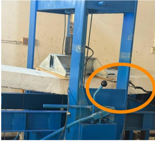
Fig. 11. Cracks developed in the concrete slab under applied load
