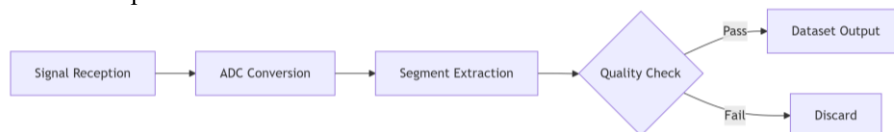
Fig. 1. Signal acquisition flow chart
