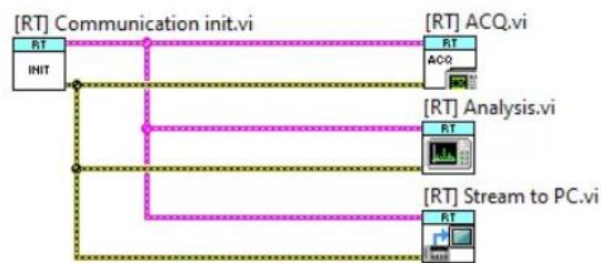
Fig. 6. Structure of a programme running on the RT operating system
