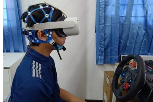
Fig. 1. The Electroencephalograph (EEG), Virtual Reality (VR) display, and the steering wheel setup on the participant during data collection
