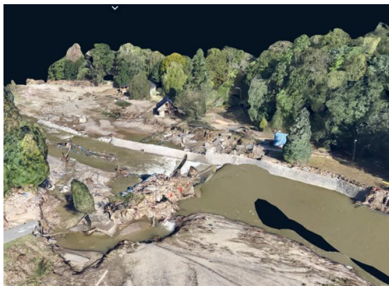
Fig. 5. 3D model created using drone imagery
