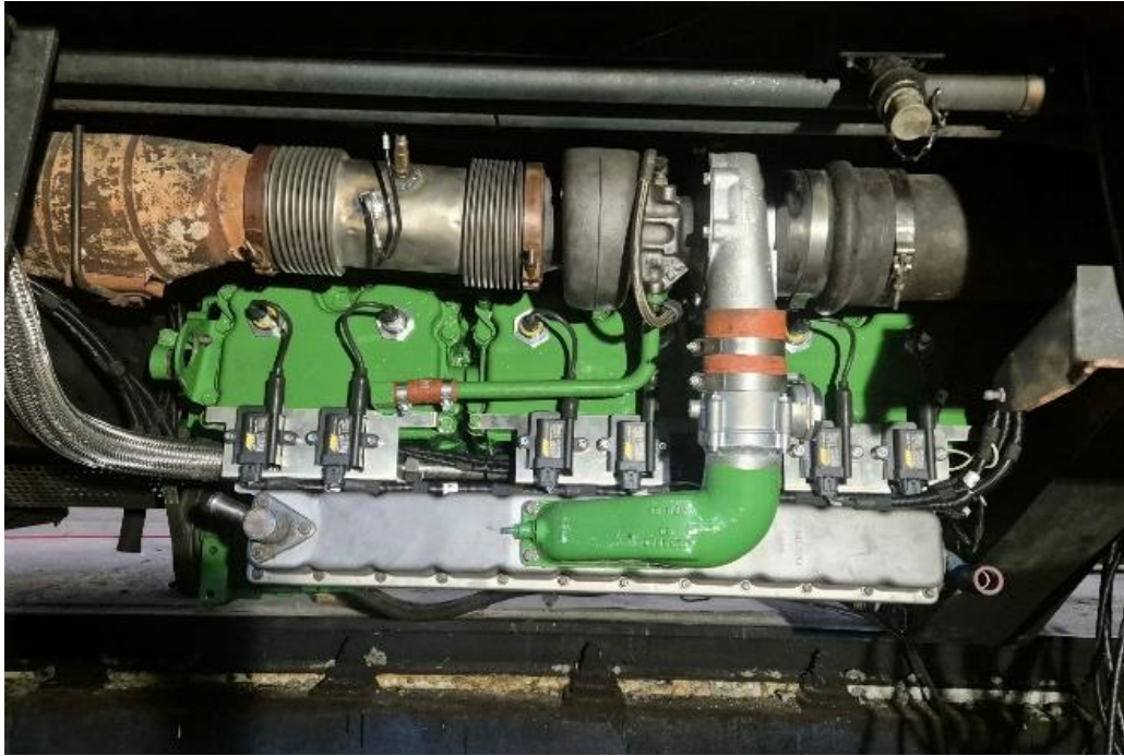
Fig. 1. Hydrogen engine installation (cylinder-head side view) on the DM'90 railcar
