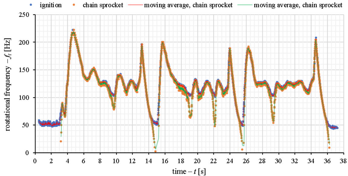
Fig. 5. Changes of rotational frequency of the chainsaw drive train components during the simulation of real operating conditions
