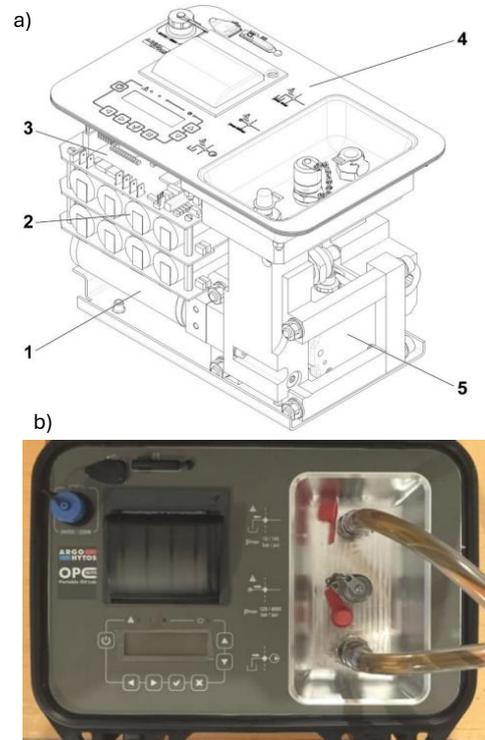
Fig. 4. a) General structure of the oil condition analyzer: 1- Engine with pump and electric gear, 2- Battery, 3- Control electronics, 4- Top side with control panel, 5- Particulate monitor, b) View of the portable oil condition analyzer OPCOMII Portable Oil Lab PPCO 300-1000 by ArgoHytos
