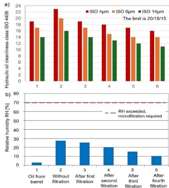
Fig. 7. Dependence of: a) oil cleanliness class according to ISO 4406, b) relative humidity RH, in subsequent microfiltration operations for the first charger
