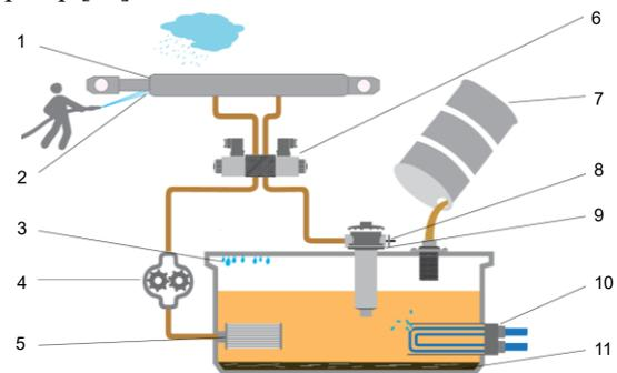
Fig. 1. Sources of contamination in hydraulic oil: 1-worn seals, 2-washing the system with water, 3-evaporation and condensation, 4-wearing mechanical elements, 5-damaged seals, 6-damaged hydraulic distributor, 7-contaminated oil, 8-lack of periodic filtration, 9-worn filters, 10-contaminated cooler, 11-sludge at the bottom of the tank [2]
