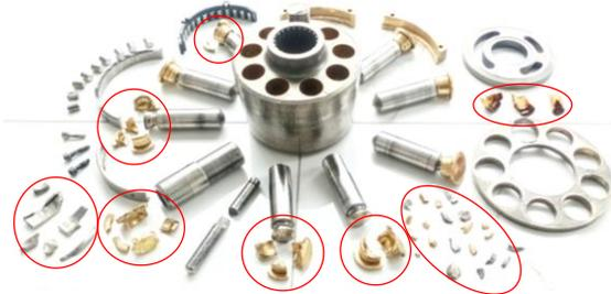
Fig. 3. View of the damaged Liebherr 566 loader multi-piston pump. Red circles mark damaged pump piston joints. [fot. S. Kołodziejcki]
