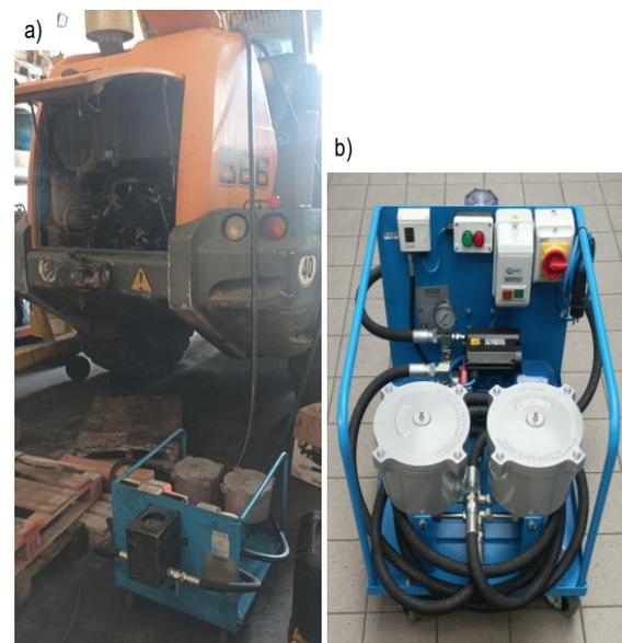
Fig. 6. View of: a) the microfiltration process of the hydraulic oil of the Liebherr 566 wheel loader on the portable Kleenoil MS2+MM5 device, 1- filtering machine, 2- hydraulic line sucking oil for filtration, 3- hydraulic line with purified oil, b) the filtering device [fot. S. Kołodziejcki]
