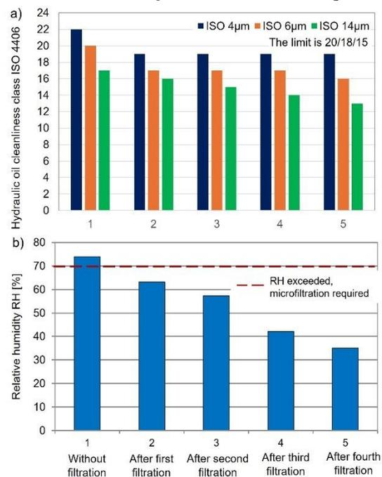
Fig. 8. Dependence of: a) oil cleanliness class according to ISO 4406, b) relative humidity RH, in subsequent microfiltration operations for the second charger
