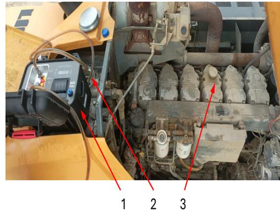
Fig. 5. View from the hydraulic oil test of a Liebherr 566 wheel loader: 1- View of the portable oil condition analyzer, 2- Hydraulic oil filler (place where the oil sample is taken for testing), 3- Loader combustion engine
