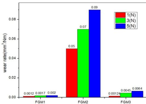
Fig. 6. Applied load effect on the wear rate of the different FGMs, N=450rpm
