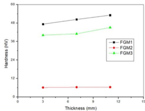
Fig. 4. The hardness of the FGMs at different thicknesses
