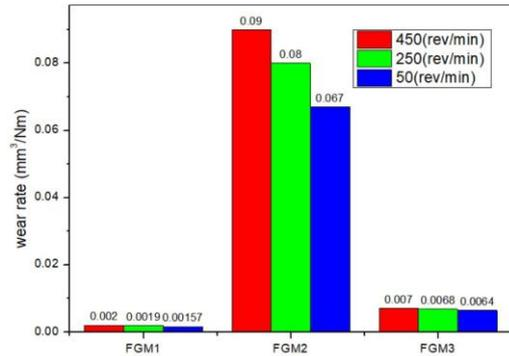
Fig. 7. The effect of the rotational speed on the wear rate of different FGMs
