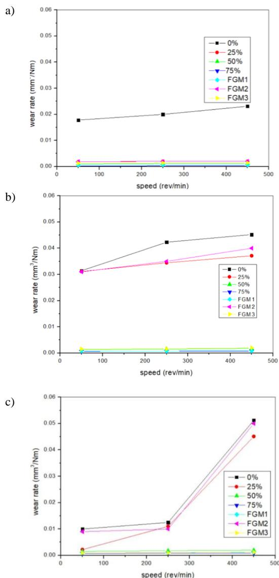
Fig. 3. Effect of rotational speed on specific wear rate of different FGMs and their layers under the applied load of 1N (a) sliding time 5minutes, (b)10min, (c)15min
