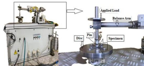
Fig. 2. Pin on disc tribometer
