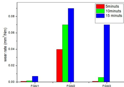
Fig. 9. Sliding time effect on the wear rate of different FGMs W= 5N and N= 450rpm
