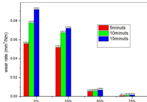
Fig. 8. Sliding time vs. wear rate of different layers. W=5N N= 450rpm
