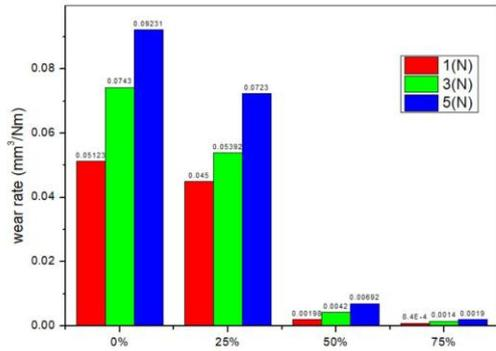
Fig. 5. Applied load effect on the wear rate of the layers, N=450rpm
