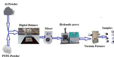
Fig. 1. Steps followed to synthesize FGMs wear testing samples
