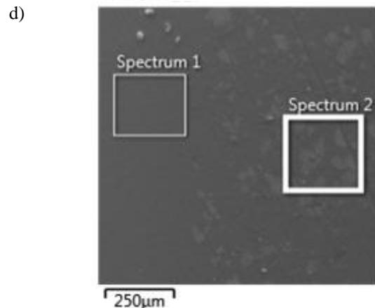
Fig. 15. EDS micrograph for the five layers FGM (FGM1) (a) EDS of the spectrum1 (b) EDS of the spectrum2 (c)Spectrum1 (d) Spectrum2
